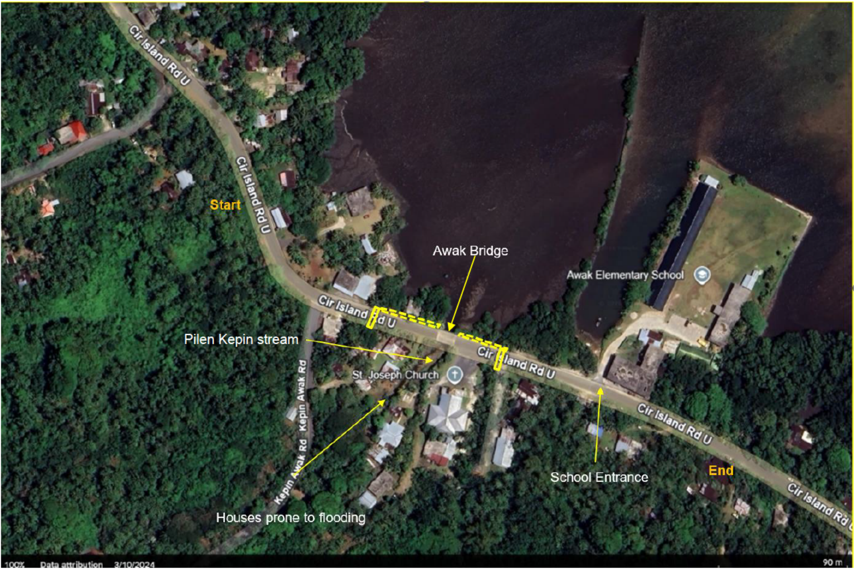
Figure 3: Location and infrastructure upgrades associated with the replacement of Awak Bridge (including nearby community receptors)
