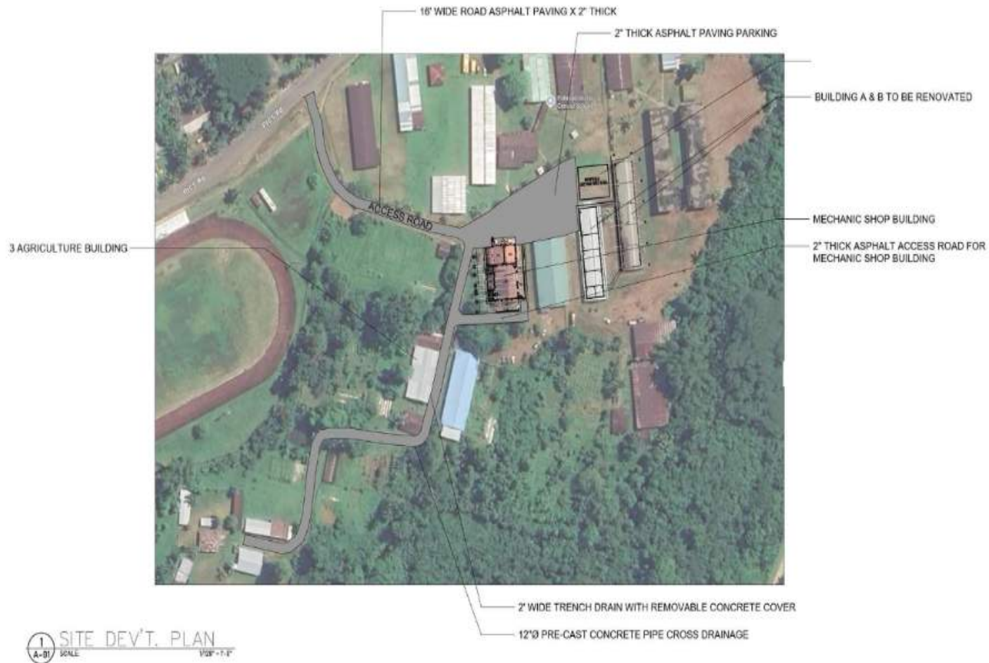
Figure 1: Layout of the proposed works
