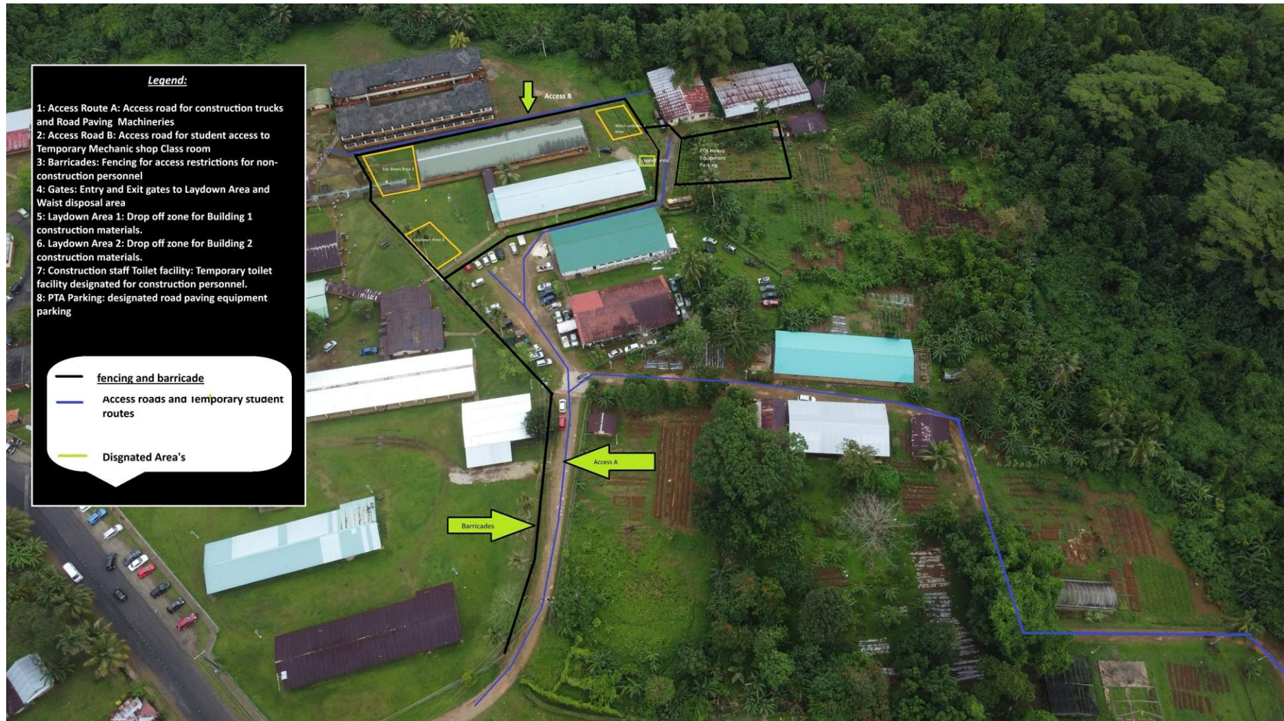
Figure 2 Traffic Management Plan & Laydown Area
